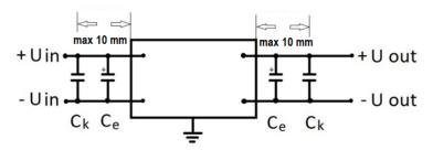
The design of the units allows their use only when mounted on a PCB. When using the units + U out with typical connection scheme it's necessary to use certain type components. In the figure: Ck – - U out ceramic capacitors of a certain operating voltage and of several μF capacity; Ce – electrolytic capacitors of a certain operating voltage and of
