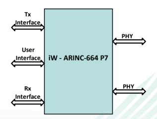
iWave's ARINC 667 P7 IP is an Ethernet Technology that provides a deterministic network to build an ARINC 667 P7 end system with guaranteed service to each subscriber with free access to the network. This protocol offers dedicated bandwidth for each node with a guaranteed quality of service. iWave offers high integrity and redundancy management, as well as UDP/IP, profiled communication layer implemented in hardware.
